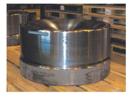
Fuel pump barrel **Certified Marking** Part No. Marking Instruction 0742843-8
