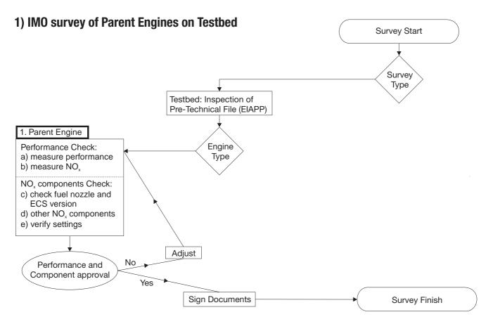
The performance parameter check is the basis of the survey methods. The measurements involved are used as reference for Member engines.
