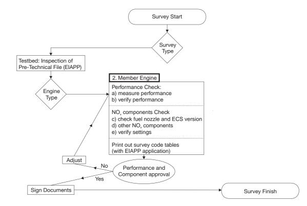
The main difference between surveying Parent and Member engines is that the  $NO_x$  emission is only being measured for the Parent engine. For the Member engine, the performance check verifies compliance based on the parent engine  $NO_x$  data.
