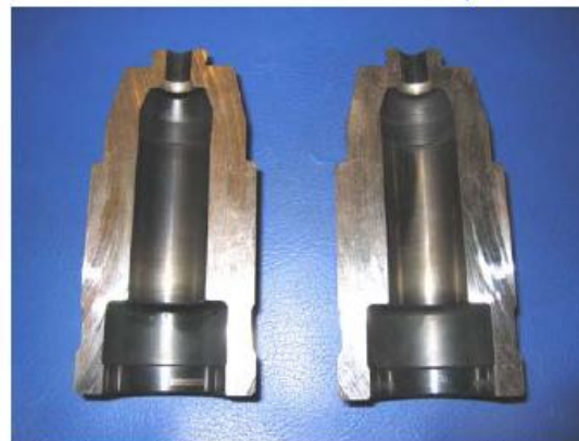
Fig.2 Spindle guide (cut open)
