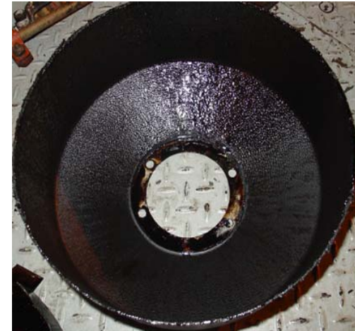
Fuel on lower surface of umbrella caused by splash from pump base bottom
