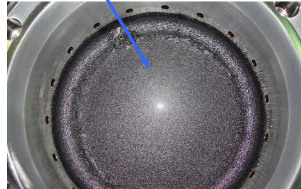
Deposit on piston crown cooling space surface
