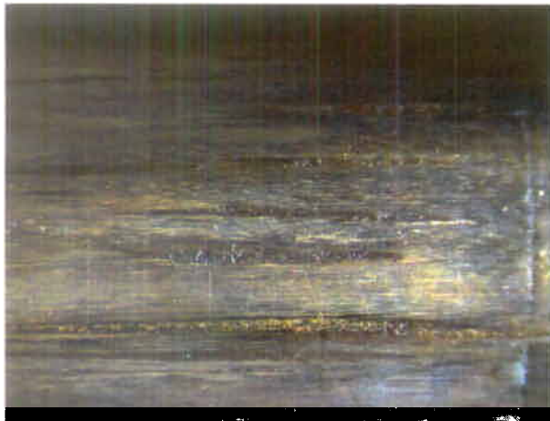
Fig. C: Further magnification of scuffing marks (7.4x)
