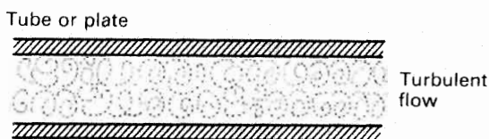
Figure 1.9 Turbulent flow of a fluid
