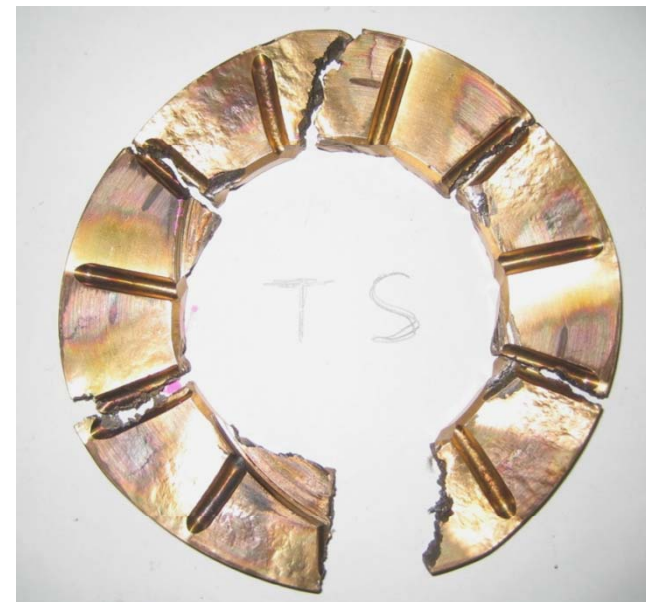
Damaged floating disc
