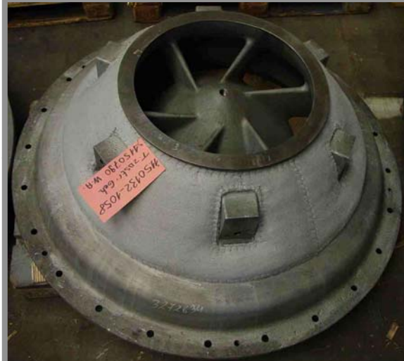
Axial admission casing with disc cooling (4-stroke)
