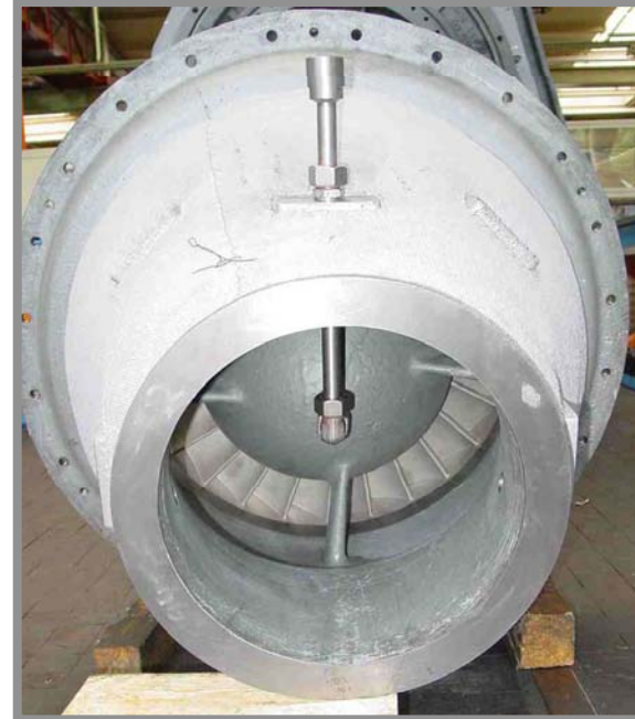
Axial admission casing with cooling pipe
