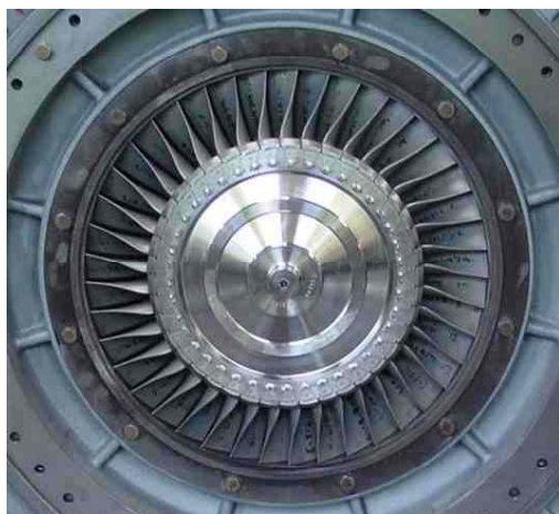
Shroud ring in outlet casing
